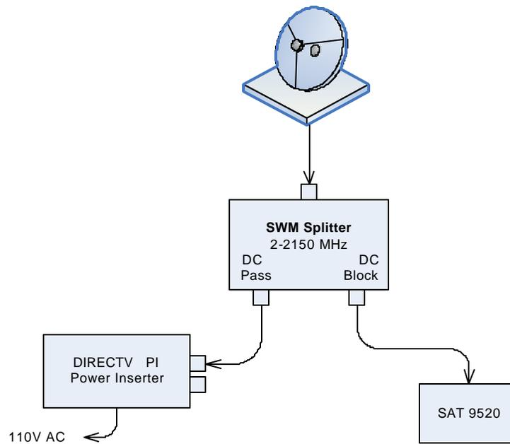
Take care when making these connections: there is a chance that an accidental application of up to 30 VDC to the SAT 9520 may damage the meter.
