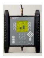
**Connections:** Coax cable connected from an output port of DIRECTV SL5 LNBF to top (SIGNAL IN) port of Super Buddy meter.
