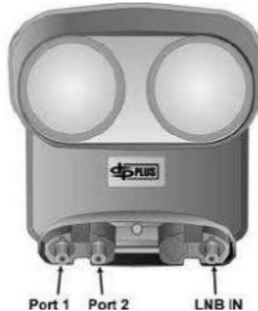
**Connections:** Coax cable connected from an LNBF output port to the XR-3 satellite meter module's ODU / LNB port
