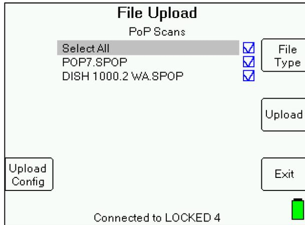
To select a file to upload, highlight it with the up and down arrows and press Enter to set the check mark. You can check as many as you like. To select all files, press Enter when the "Select All" row is highlighted.
