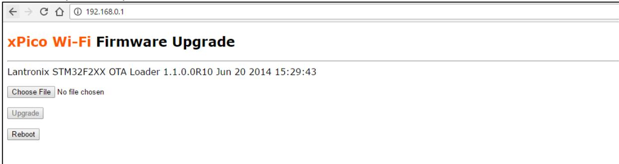
5. Click upgrade and wait for the upgrade to finish. It should say “Upgrade successful” and allow you to reboot the device. After clicking Reboot and OK, the upgrade is finished. A “Please wait” screen will be displayed while the Wi-Fi module resets and an attempt to reconnect is made. The reconnect will most likely not be successful, but that is OK.
