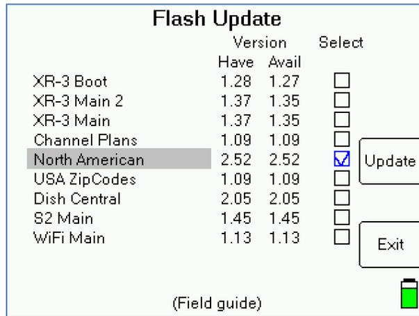
When you have the desired components selected, press Update. The meter will begin downloading each component and will display a progress bar for each.
