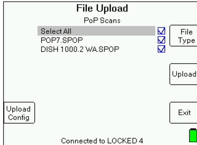
This screen lets you select which files to upload. Only one type of file is displayed at a time. You can upload several files of the same type at once. If you have several types, you will need to upload them in batches, with each batch containing files of the same type.
