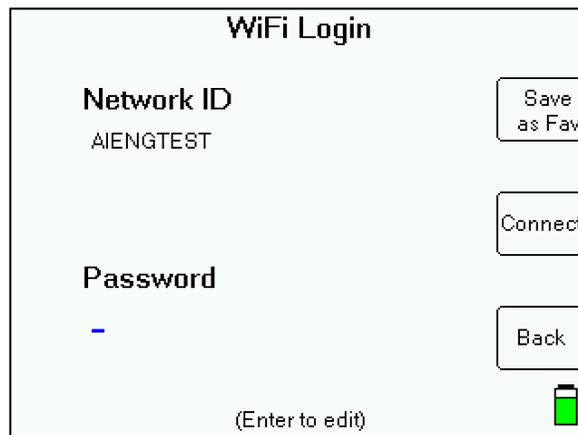
To enter a password, first press the Enter key. An on-screen keyboard will appear.
