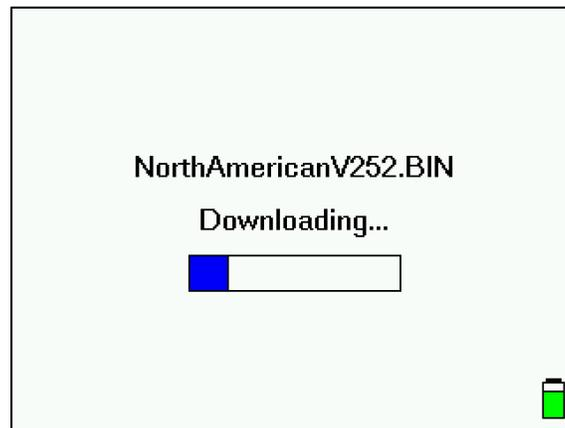
The download process can take up to 8 minutes to complete, depending on the number of components that need to be updated. When complete, the meter will reboot and default back to the main Run screen.
