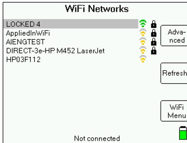
The network name being broadcast (SSID), signal strength indicator, and encryption status of each Wi-Fi network are displayed.
